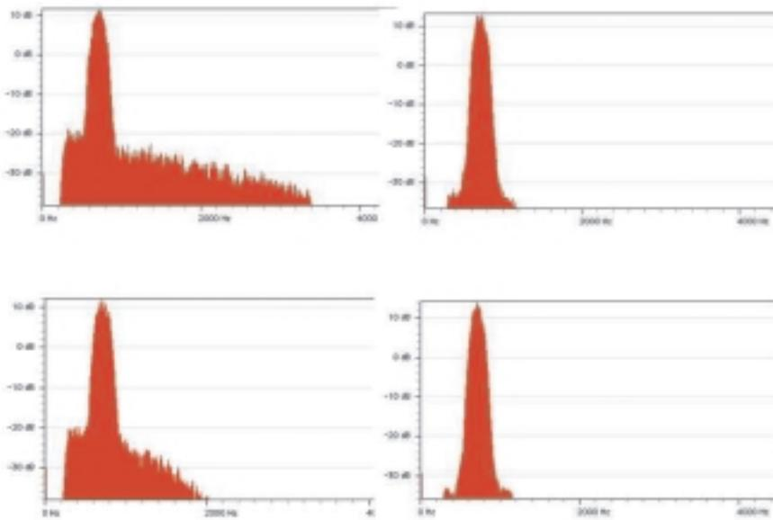
Audio spectra of typical HF noise taken with 250 Hz Xtal filter. Top to bottom as follows:
